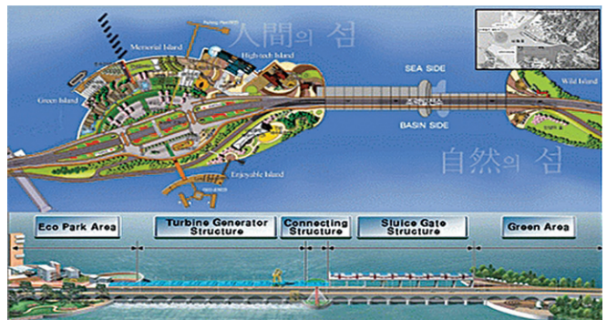
Fig.1 Plane view of Sihwa tidal power plant
